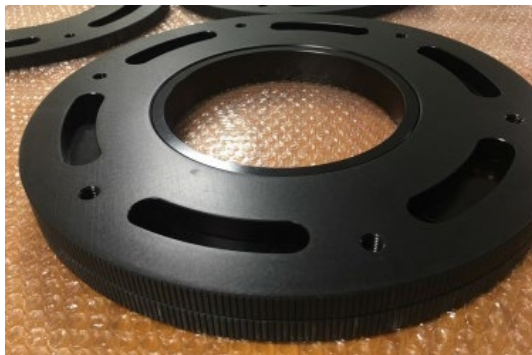
Customized aluminum plate allowing for precise positioning of the antenna
