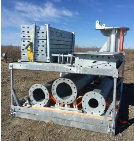
Foundation & pole on custom pallet
