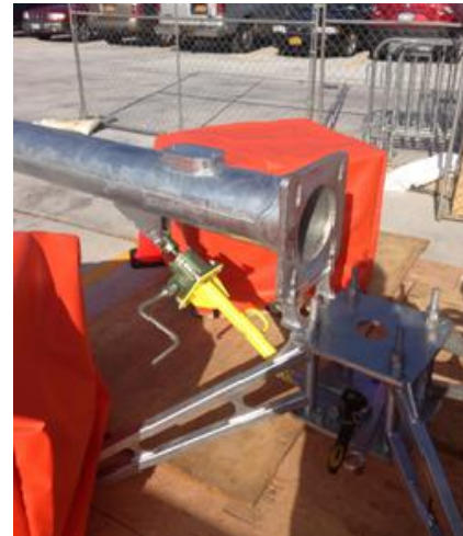
Tower Raising System
